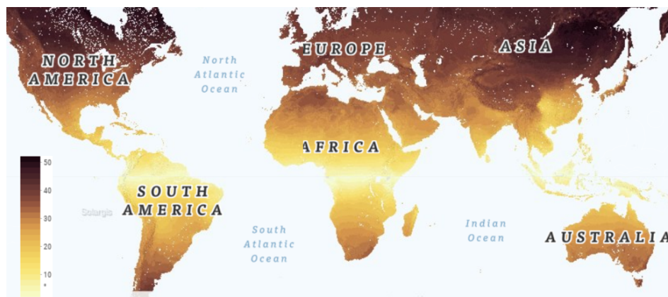
Figure 3.14: Optimum tilt angle for PV panel modules
