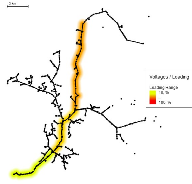
(p) Line loading after V Etapa load connection.
