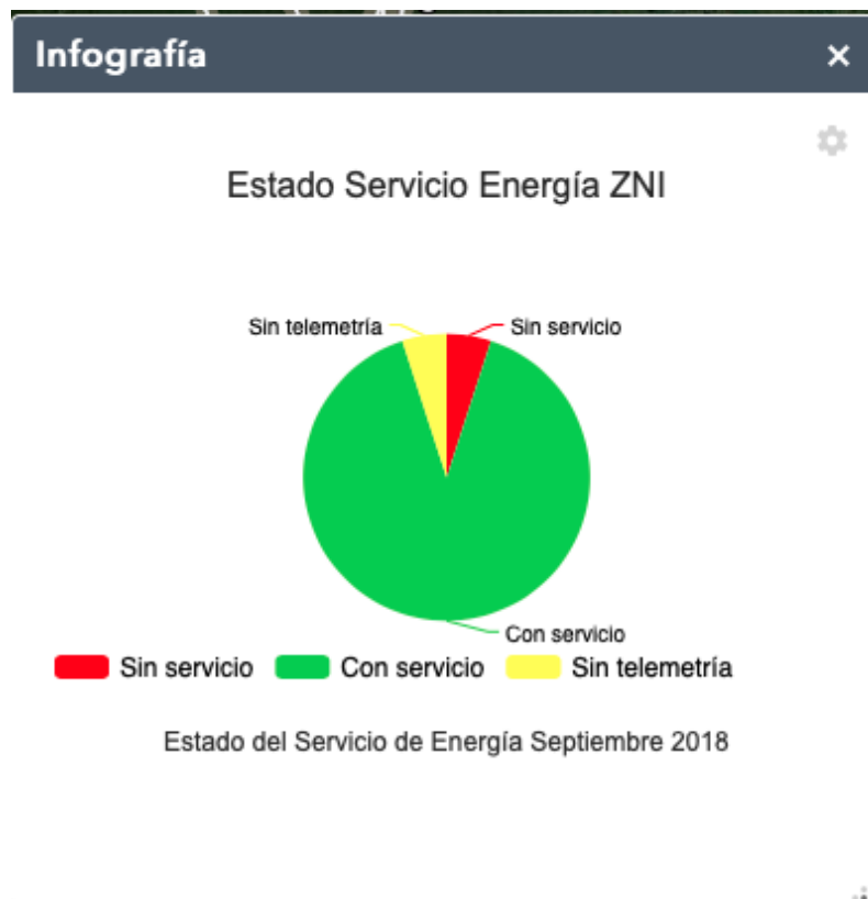
Figure 3.7: Convention used and proportion of users provided with service of electric energy. Green users means with electrical energy and telemetry service. Red user means those user without service, and yellow users means those users without of telemetry.
