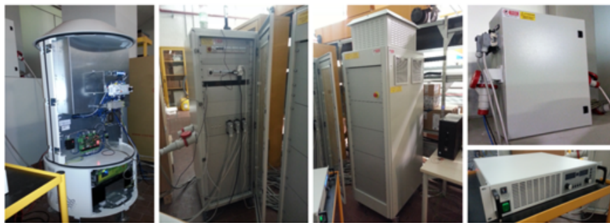
Figure E.2: Devices of the Lab IoT for the test bench: (from left to right) ESS, CompactRio controller, resistive load, (top) portable measurement device, (bottom) DC power supply.
