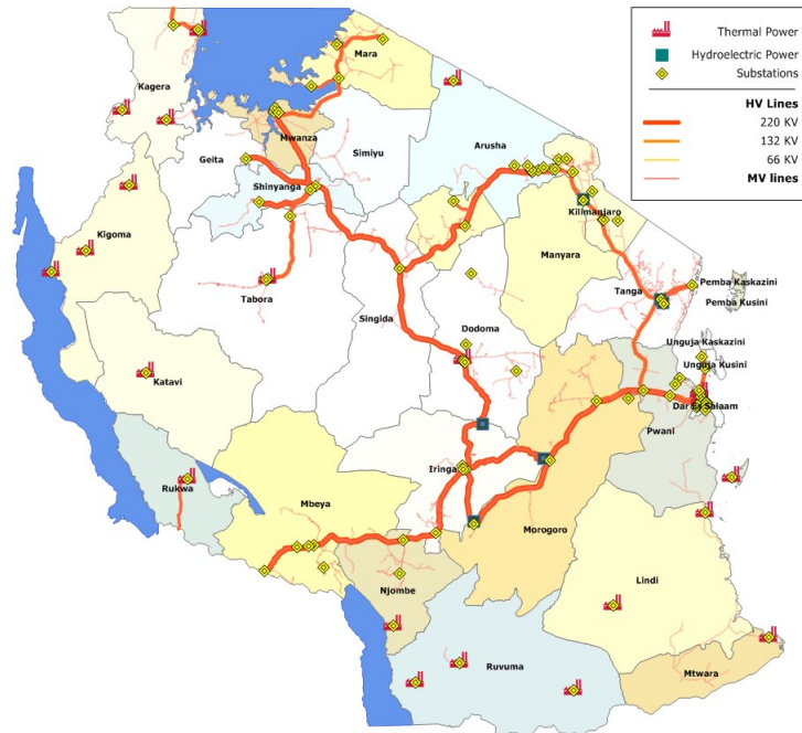
Figure 3.6: Tanzania existing grid power network.
